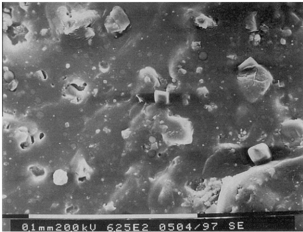
Fig. 1. SEM photograph of Eurobitum bituminized radioactive salts. Both smaller ( \varnothing 2\text{--}3\ \mu\text{m} ) and larger ( \varnothing 15\text{--}20\ \mu\text{m} ) \text{NaNO}_3 crystals, as well as other salts, precipitates, and (hydr)oxides, are homogeneously dispersed in a matrix of bitumen. Note that the bitumen matrix is almost 'saturated' with the waste substances. Energy-Dispersive X-ray (EDX) analyses show that even the places that apparently consist of 'pure' bitumen contain \text{NaNO}_3 and \text{CaSO}_4 .
